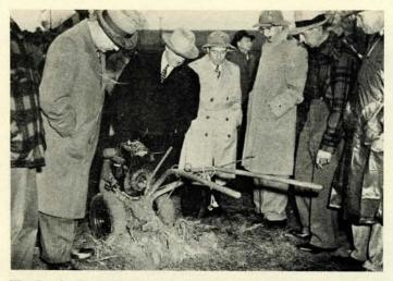
The *Duplex Rototiller* (shown above with hood removed for the demonstration) was presented to the dealers at the 1950 Field Days. Having two tiller units which rotated simultaneously in opposite directions, the *Duplex* was over 25 years ahead of its time and was too much of a novelty to win wide acceptance.
