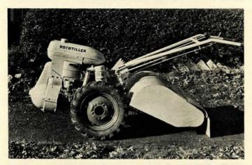
The Graham-Paige Rototiller was modeled after the B1-3 built in Troy. Graham-Paige was licensed to manufacture these large machines according to Rototiller designs. The original Rototiller company then converted to the manufacture of smaller machines for home gardeners in 1945.
