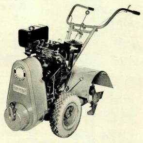
Only a very few of the *Model 5* tillers were made in 1956 and, unfortunately, none remain in original condition now. They were unique in that the tine and hood assembly was removable for the attachment of other powered accessories at the rear of the machine.
