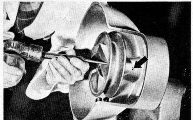
FIG. 30—DRIVING CLEVIS PIN INTO HOUSING
