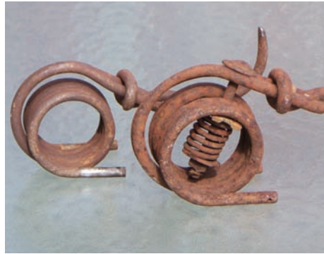
Graphic F— 1937 Rototiller, Inc. Model B1-3 two piece spring tine w/Booster insert. The extra spring indicates a need for additional tine strength due to different soil conditions.
