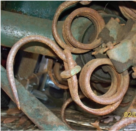
Graphic E—1937 Rototiller, Inc. Model B1-3 two piece Spring Tine.
