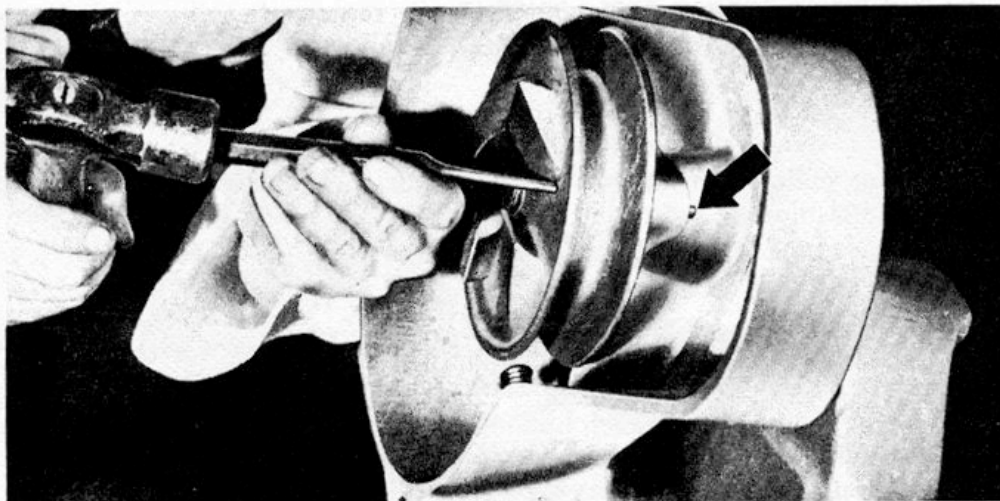
Figure 20. Driving Clevis Pin Into Housing
