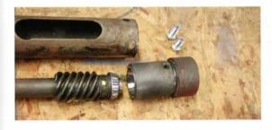
The rear bearing and the spacer next to it also wear. I have replaced the rear bearing with a new one or a good used one from the front position of a parts machine. When the shaft is assembled into the tube, there should be little to no noticeable endplay on the shaft. If there is excessive endplay, you will need shim washers between the spacer (noted with the yellow dot) and worm. There also may be shim washers between the bearing and rear snap ring to limit endplay of the shaft.
