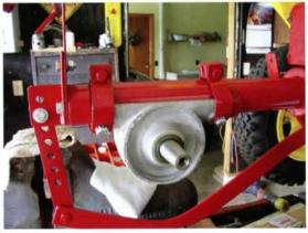
I have not done much to the engine other than clean it up and rebuild the carburetor. Eventually I will install new rings and have bushings installed in the crankshaft bores in the engine case, as there is more slop there than I like. The engine is a Briggs & Stratton model 8B, which is the first aluminum engine. 🚜
