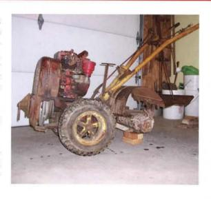
than getting one from another machine, I don't have a source for a new one. The brass worm gear is very easy to access by removing the four bolts that attach the aluminum gearbox to the main tube.
