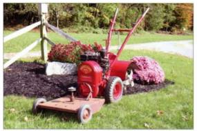
Mower attached to the "Lightning Change Front". Unfortunately, it is missing the gearbox that drives the blade that mounted in the left corner near the front of the tiller. In the photo below you can see there is a difference in the hood arrangement over the tines. My 1957 Model 3 has an adjustable flap called the Tiller Hood Depth Regulator. This was new for 1957 and it seemed to me more of a bother than it was worth.
